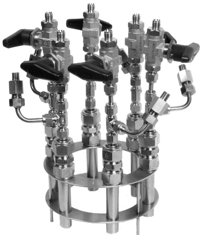
Fig. 6. Multiplex-reactor consisting of six pressure reactors and a frame for heating in an oil bath.
